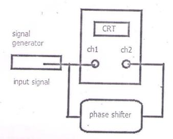
As shown above, the input coming from the signal generator is connected to the ch1 of the cro as well as to the input of the r-c n/w.
