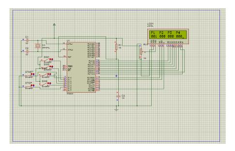
nConclusiuThus, a Electronic Vothing Machine using AT89C51 was on: simulated using proteus with the help of keil. The results of voting were virtually verified using LCD in proteus.
